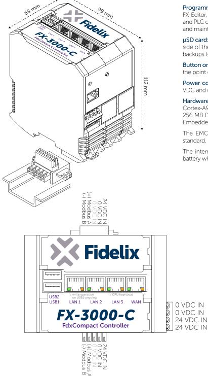
**Networking:** The controller has one Ethernet port, marked 'WAN', to connect the controller to an external network. The three other ports, marked 'LANx' can be used to connect a VISIO-15-C touchscreen display, extend the local network, connect multiLINK modules, or to connect field devices. All ports operate at 10/100 Mbit/sec and have automatic speed negotiation (MDI/MDI-X). The built-in router operates fully independent and offers IEEE 802.1X support.
